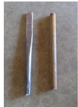
Mild steel hammer and Mike's style of punch.
