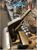
The filling vise is an insert that fits into your post or bench vice. As the name suggests, it holds the stock at an angle, allowing easier filing. The Cloverdale Forge filing vise allows the user to grip multiple thicknesses of material and tapers, adding versatility to your shop bench.
