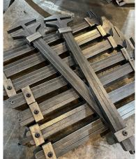
Blacksmiths typically need various bending fork sizes for shop work, including those that will work within a tight radius and forks which move larger stock sizes. The adjustable bending fork provides multiple tools in one, replacing the need to buy or make multiple forks for your toolbox.
