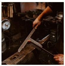
Hot Square sets allow users to check their work for squareness efficiently and safely while working with hot material. The square handles are approximately one foot long and come in 45\*, 90\*, and 120\* degree angles. The 45 degrees also included a removable center finder for up to 10".
