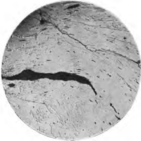
FIG. 47.—Cracks in a boiler plate which gave way when being tested under water pressure. This section was cut close to the point where the plate failed at a crushed and distorted rivet hole. (Stead.)
