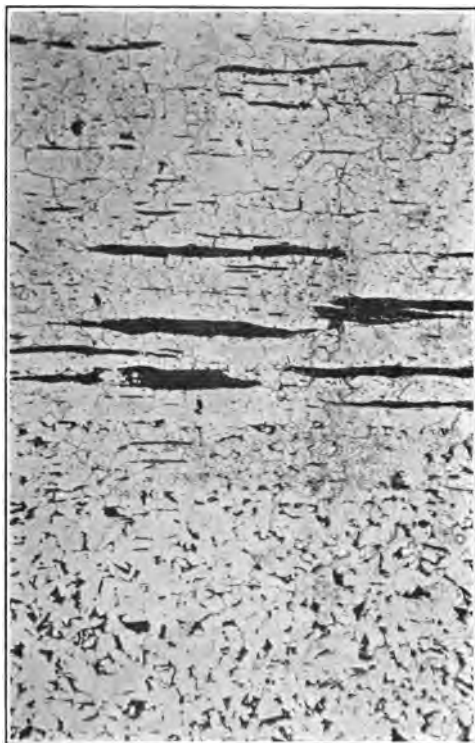
FIG. 18.—A longitudinal section of a bar made up of alternate layers of wrought iron and soft steel. Magnified 40 diameters.
