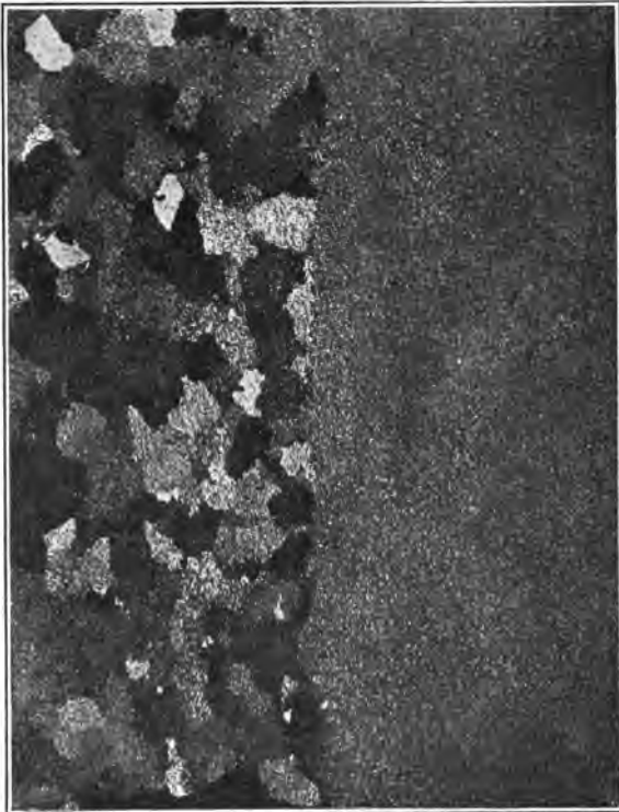
FIG. 32.—A piece of grossly crystalline soft steel sheet completely refined on the side which was reheated for a few minutes to about 1000° C. (Full size.)
