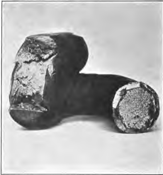
FIG. 16.—A piece of wrought iron showing that it is possible to obtain a fibrous and a crystalline fracture in the same piece of good material.
