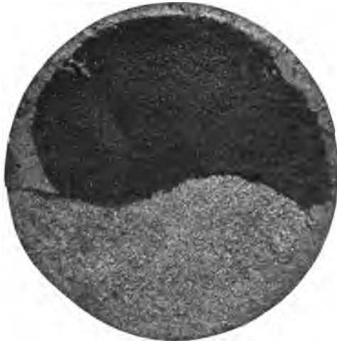
FIG. 39.—Fracture in cast tool steel. The dark portion at the top became blue in colour during tempering, thereby revealing the presence of an initial crack. The lower portion and the outer edge all round the top finally broke out of the solid.
