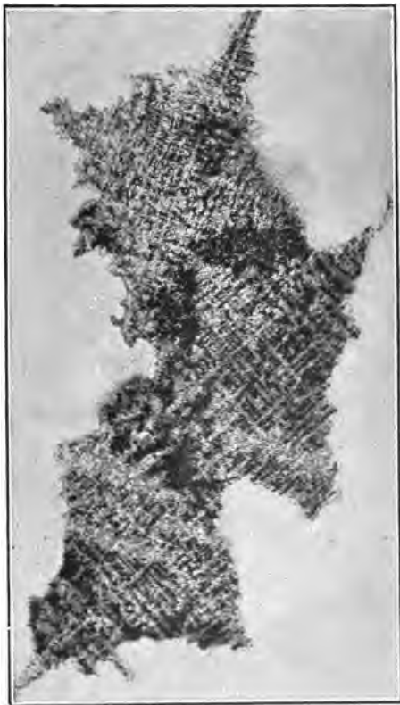
FIG. 21.—Sulphur print of a cross-section of three crystallites from a large steel ingot, showing the white skeleton crystals with sulphur trapped between the branches. Natural size. (Stead.)
