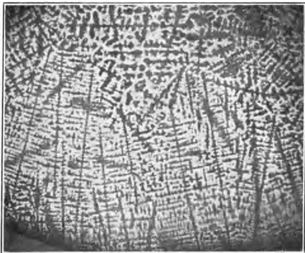
FIG. 22.—Steel rich in phosphorus. A cross-section polished and developed by a new reagent for revealing the position taken by phosphorus. The dark parts are the primary crystallites free from phosphorus. The light parts are rich in phosphorus. (Stead.)
