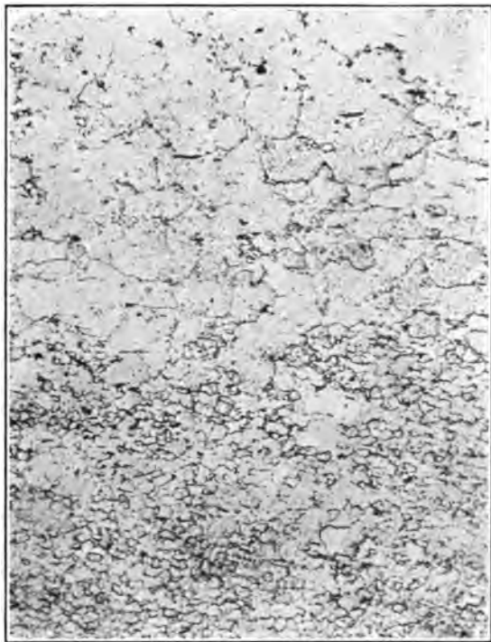
FIG. 42.—Portion of soft steel ring which was annealed at a low temperature after being cold-strained. The top portion, which represents the edge of the ring, shows growth of large crystals. Magnified 60 diameters.
