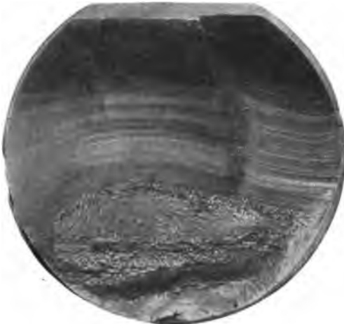
FIG. 31.—A fracture of a steam-hammer piston rod which broke while in use.
