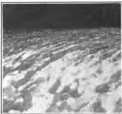
FIG. 45.—Surface of a forced drill hole. (Stead.)
