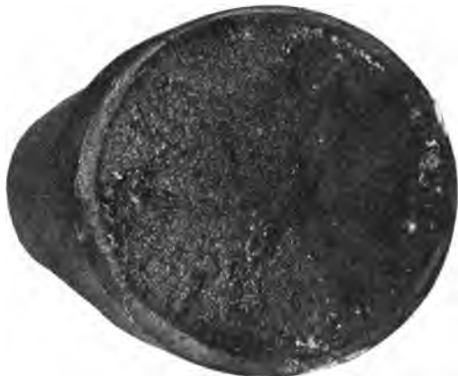
FIG. 38.—Broken lathe centre showing refined outer zone, coarse centre portion, and blue circular part at right-hand side.
