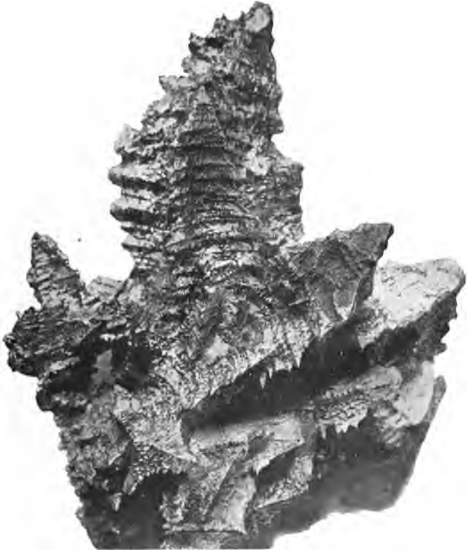
FIG. 20.—Crystallites from a cavity in a large steel ingot. Natural size. (Stead.)
