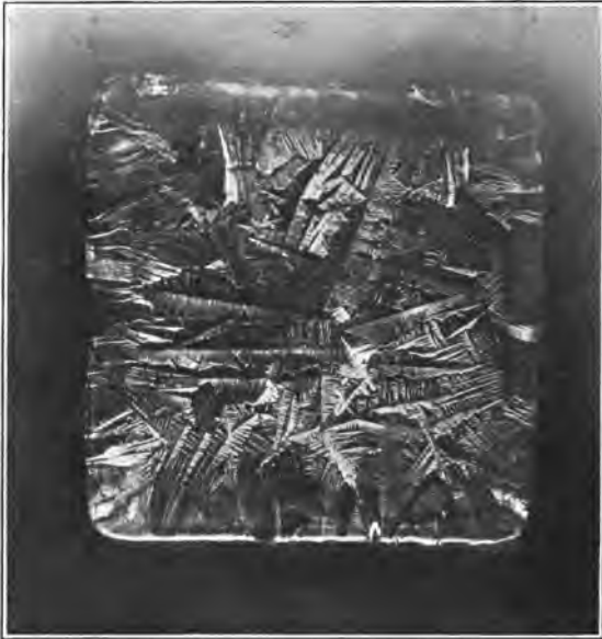
FIG. 19.—Surface of an ingot of antimony showing the fir-tree-like formation of crystal.
