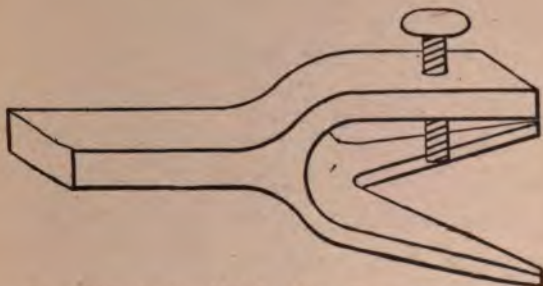
"Apprentice's" Device for Holding Tire-Bolts. Fig. 105—General View of the Tool.
