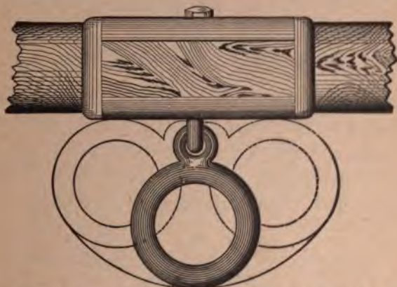
Making a Staple and Ring for a Neck Yoke by the Method of "M. D. D." Fig. 32—The Finished Ring.
