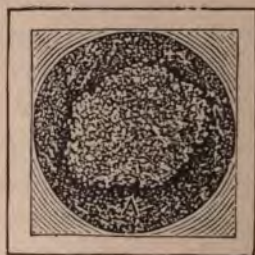
Fig. 161—End of Broken Axle, Dark Portion Showing Old Crack.
