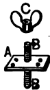
Fig. 144—Showing the Iron Parts for the Other End of the Gauge Bar.
