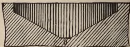
Fig. 91—Showing another Improper Way of Grinding.
