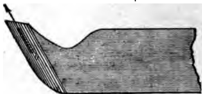
Fig. 140—Showing the Rake of the Bottom Face.
