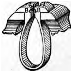
Fig. 162—Showing the Device adapted for Holding Round Pins.
