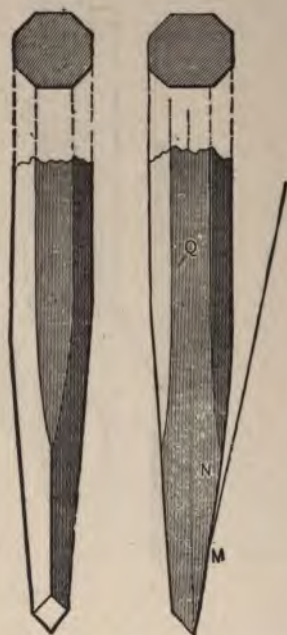
Fig. 57—The Diamond Point Chisel for Shallow Work.
