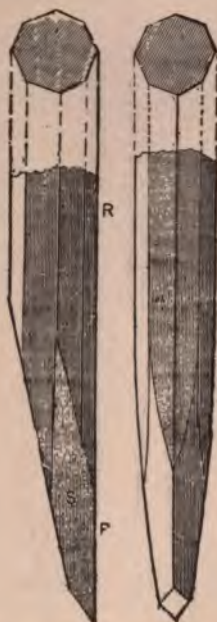
Fig. 58—The Diamond Point Chisel for Deep Work.
