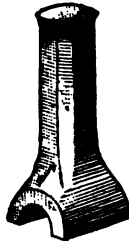
Fig. 103½—Old Method of Forging a Swage.
