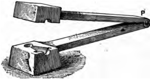
Fig. 112—Hinged Dies for Forging Fig. 111.
