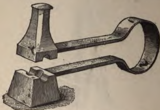
Fig. 106—Shows a Spring Swage for Light Work.
