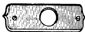
Fig. 190—Piece of Wood used to Secure the Knife in its Place and Admit the Tap.
