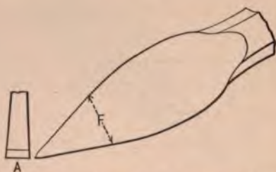
Fig. 65—A Better Shape for Cold Chisels.
