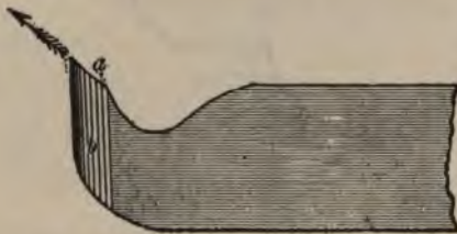
Fig. 139—Showing the Rake of the Top Face.
