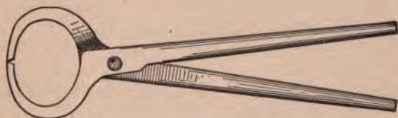
Fig. 128—Showing a Faulty Method of Making Pinchers.
