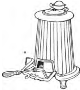
Figure 39.—Cast Iron Firepot.
