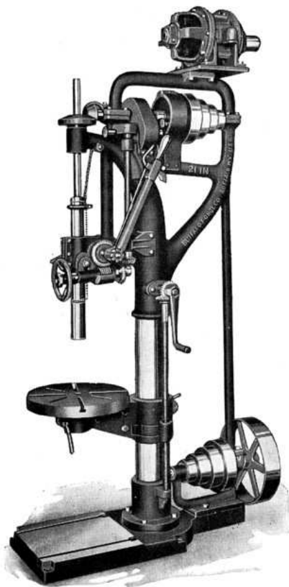
Above illustration shows standard motor drive arrangement.
