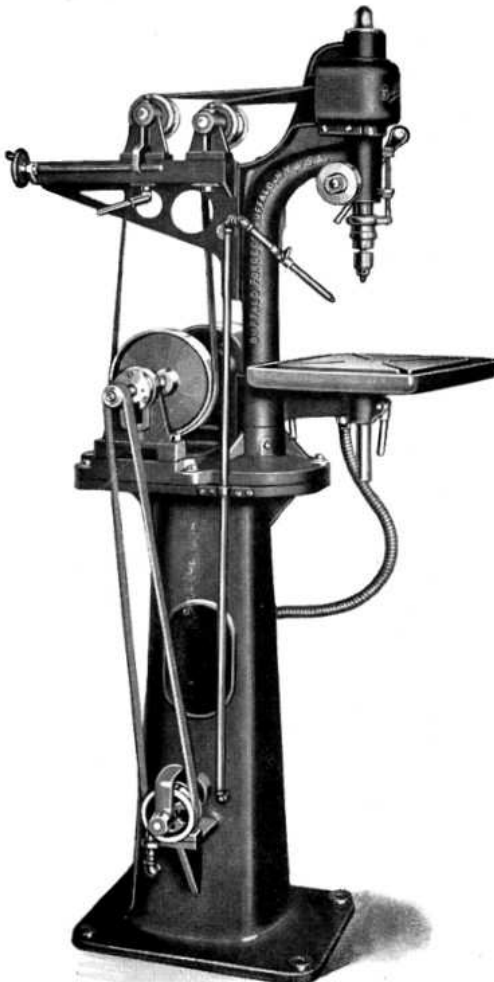
Recirculating pump for cutting compound furnished at extra cost.
