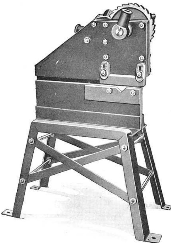
No. 23 Slitting Shear. Can also be furnished without stand.
