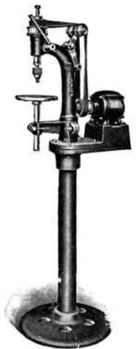
"Buffalo" 10" Junior Bench Drill mounted on Pedestal. Furnished only when ordered. Extra charge.
