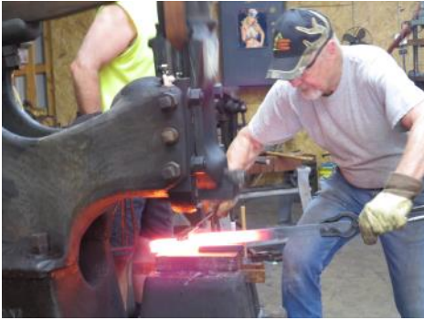
Bernie putting the offset in the jaws. The bars were welded together on the ends and shaped and bent at the same time.
