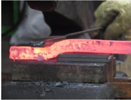
Bernie putting the offset in the jaws. The bars were welded together on the ends and shaped and bent at the same time.
