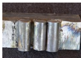
Tool to give three points of contact in a vise. 1/2" rounds welded to a piece of angle iron.
