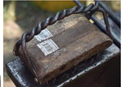
Bryan made this brush by gluing 3 brushes together and making a new handle.
