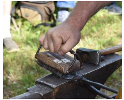
Bryan made this brush by gluing 3 brushes together and making a new handle.
