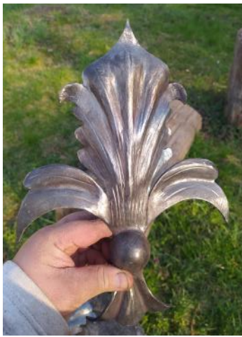
. Floral elements are 3 mm thick sheet that is embossed and stamped.
