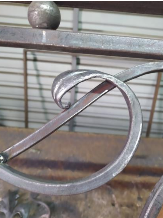
. Floral elements are 3 mm thick sheet that is embossed and stamped.
