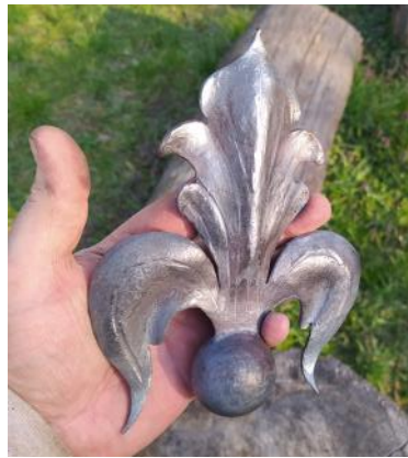
. Floral elements are 3 mm thick sheet that is embossed and stamped.
