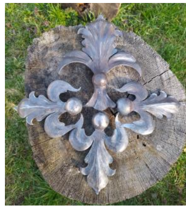
. Floral elements are 3 mm thick sheet that is embossed and stamped.
