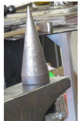
His cone mandrel fits his Hardy hole and has a key to lock it in place.
