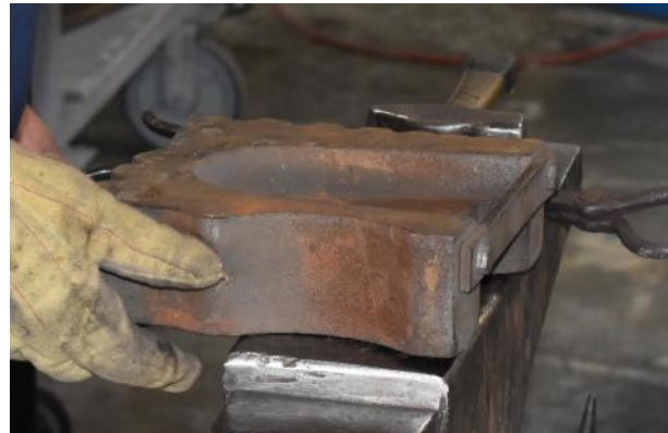
Bob's Swage block has a piece of flat bar bolted across the opening of the shovel blank. This keeps the blank from sliding out when forming it. It also makes a nifty carrying handle.
