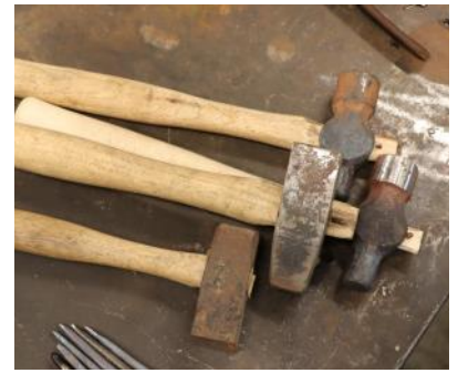
Flatters and set hammers. The Ball peens round ends were reshaped and softened so they could be struck with a hammer.
