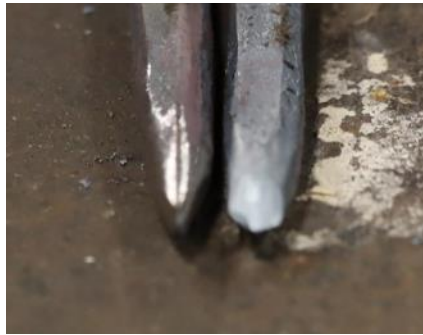
Slitting Chisels. These are small so they will heat up and deform quickly. Keep them cool while using and be prepared to sharpen often.
