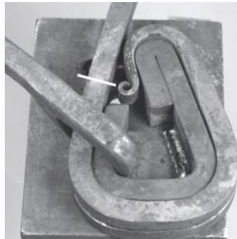
A test piece was made to calculate the length of stock required for the handle
