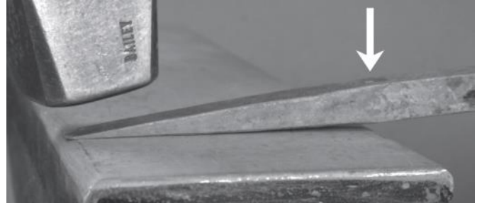
A test piece was made to calculate the length of stock required for the handle
