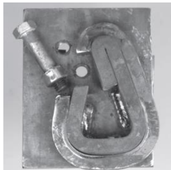
Here the D-shaped jig is welded to a base plate and a spacer bar fitted
