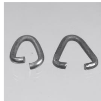
The clip after being cut from the mandrel.
