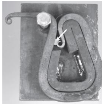
The material covers the location of the first pin
