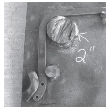
A jig for the blade cam bar showing a 2-inch ID bend
