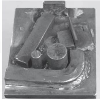
The Alpha jig with stops & spacer bars fitted
