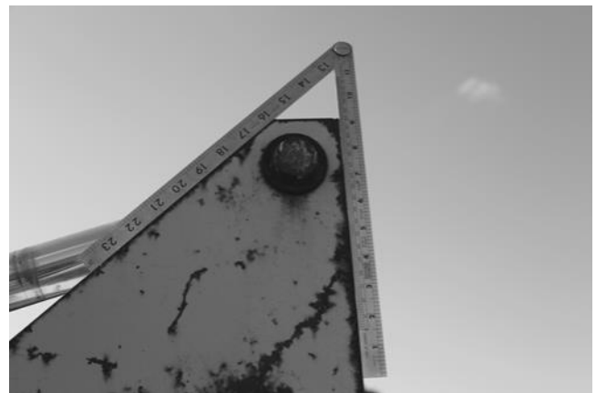
To measure an angle using the Line of Chords, first set the leaves of the rule to match the angle to be measured. In this case, a steel plate.
