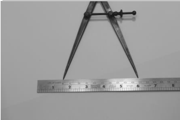
The divider setting is transferred to the Line of Chords scale to directly measure the angle. In this case 49°.
