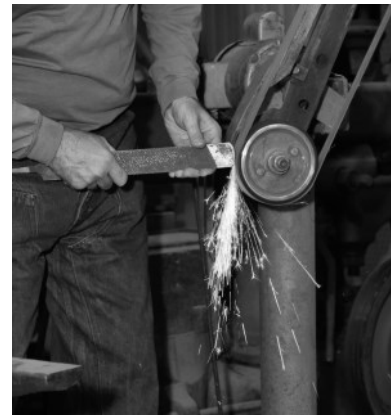
Ken demonstrates a spark test at the November Meeting.
