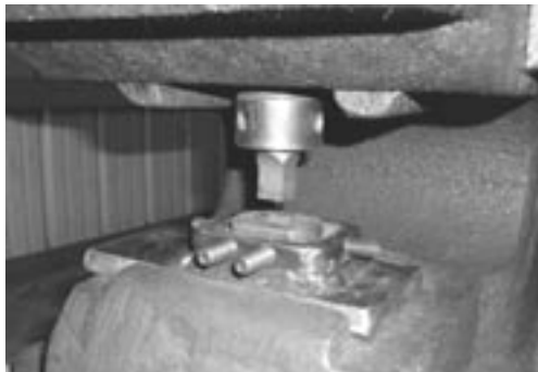
Two views of the die holders and the stripper cage
