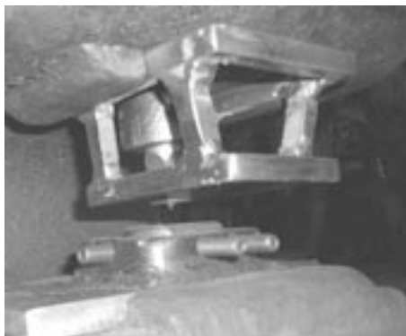
Two views of the die holders and the stripper cage
