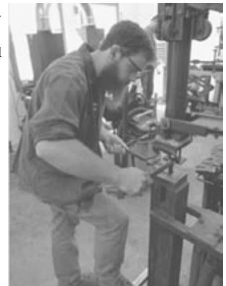
The author splitting a piece of steel under the treadle hammer.
