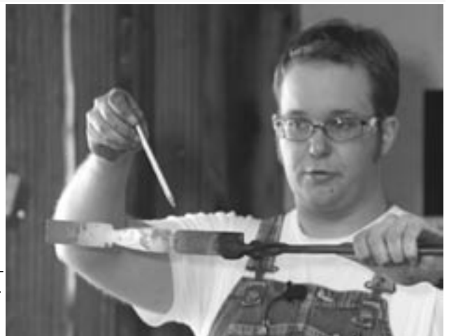
Right, Both fullers are done, starting to narrow down the center section.
