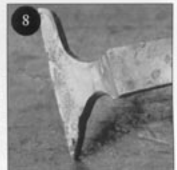
Using 1/2" fuller under the horn and 3/4" fuller under heel, fuller waist to width
