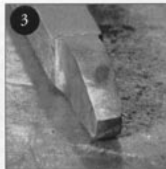
Flatten material in front of fullered groove to approximately 1/2" thick
