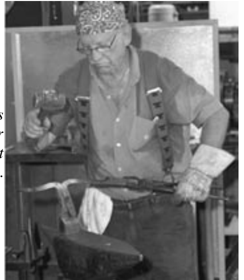
The first split is driven down over a hardie to start opening it.
