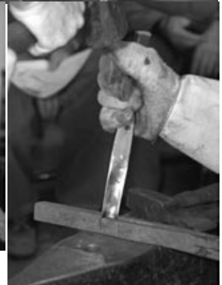
The second split starts in the middle and overlaps the first cut. A curved chisel is used to transition from the cut to the face of the bar.
