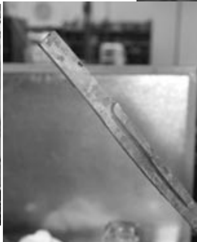
The second split starts in the middle and overlaps the first cut. A curved chisel is used to transition from the cut to the face of the bar.
