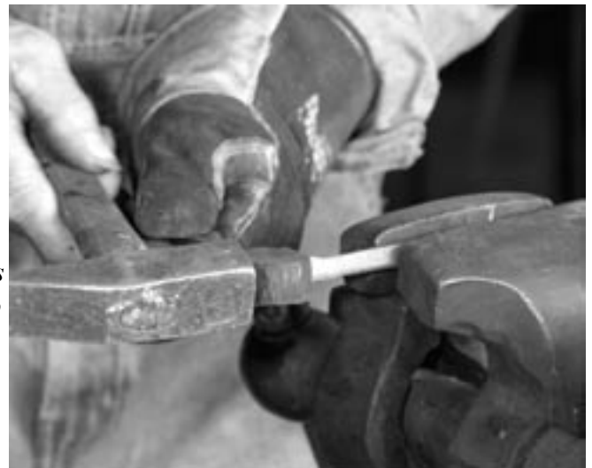
A Monkey tool is used to clean up the shoulder on the tenon.
