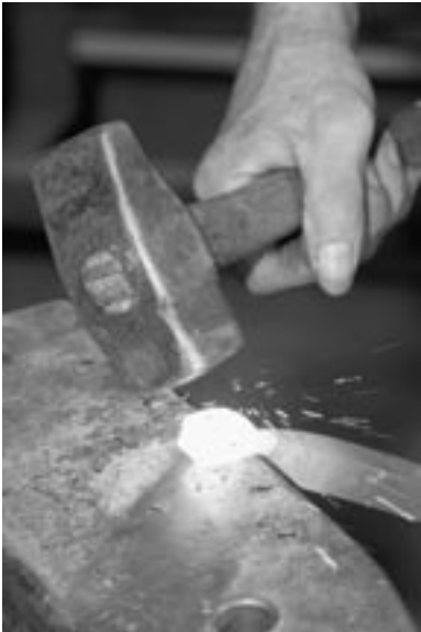
The hanger is started with a disk on the end of a bar.
