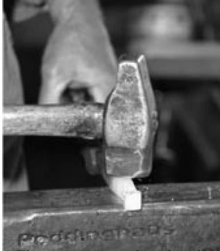
The taper is started on the edge, leaving a blob for the tenon.
