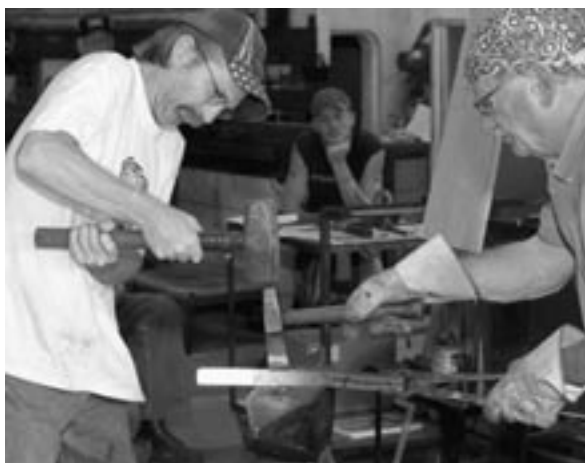
The second split starts in the middle and overlaps the first cut. A curved chisel is used to transition from the cut to the face of the bar.
