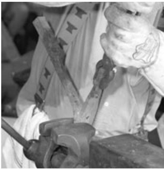
The split is starting to open. Lou uses a real thin chisel to cut the web that connects the two sides of the cut.
