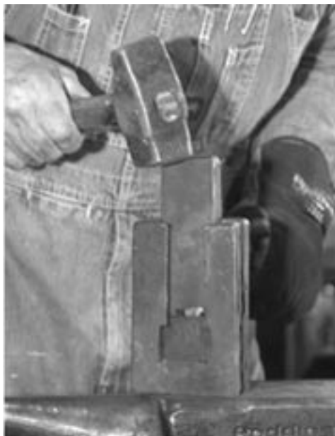
The tenon is formed using a Smith'n Magician type tool. Note: the top die has a notch cut in it to control the diameter of the tenon.
