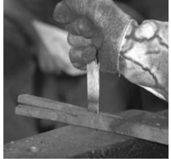
The split is starting to open. Lou uses a real thin chisel to cut the web that connects the two sides of the cut.
