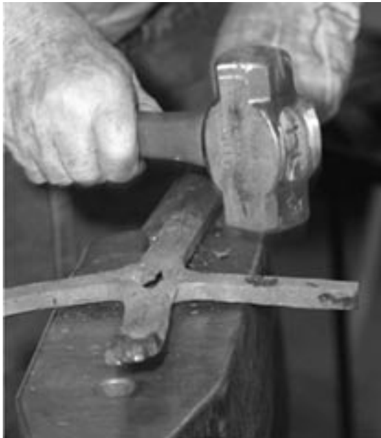
Lou finishes opening the cross on the anvil by hammering it flat.
