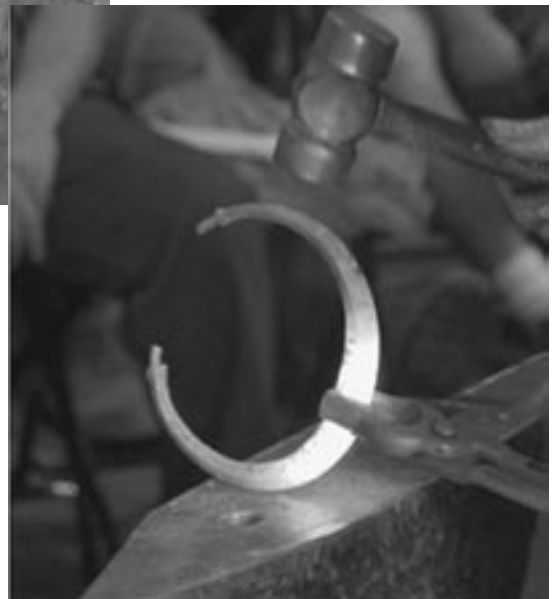
When forming into a ring, Walt makes sure that the support and where he hits it, are on the flats to preserve the sharp corners on the piece
