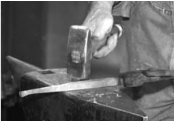
Once he has the length he wants, the taper is cleaned up.
