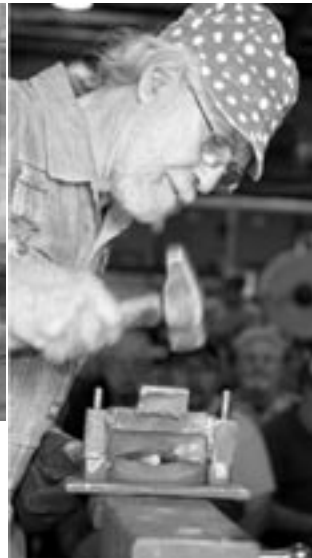
The tenon is formed using a Smith'n Magician type tool. Note: the top die has a notch cut in it to control the diameter of the tenon.
