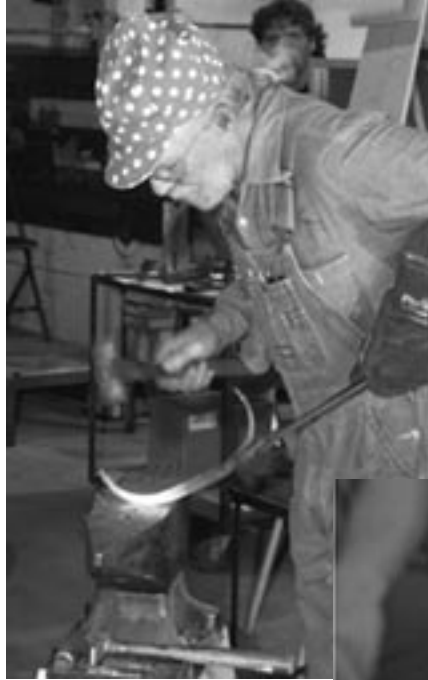
When forming into a ring, Walt makes sure that the support and where he hits it, are on the flats to preserve the sharp corners on the piece
