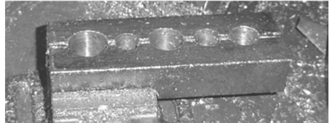
The bundle is drilled and chamfered
