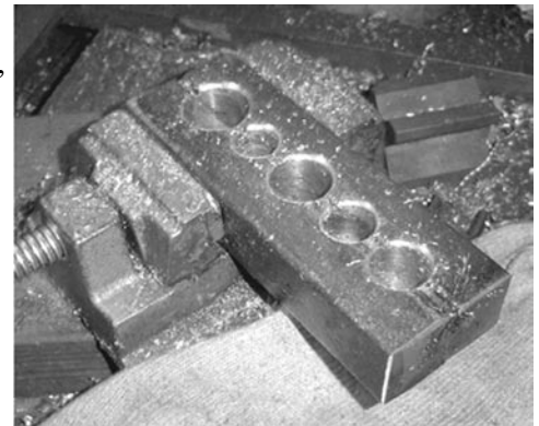
The bundle is drilled and chamfered
