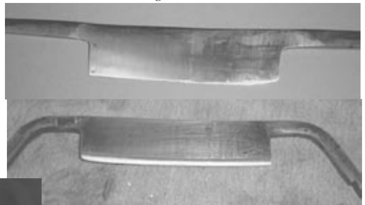
Above, Etched, sharpened, and the handles bent
