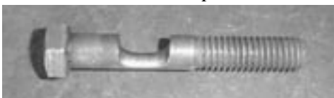
Above, Treadle control linkage. Below, worn out pivot bolt
