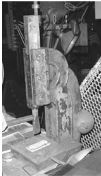
Below and right, My kick press which has a similar die/ram set up as the fly press, but is foot operated instead of having a screw.
