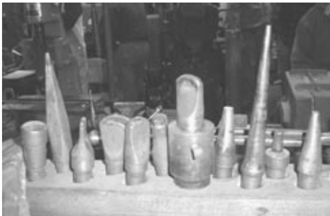
Below, Phil's press tooling, note the top die extender in the middle.
