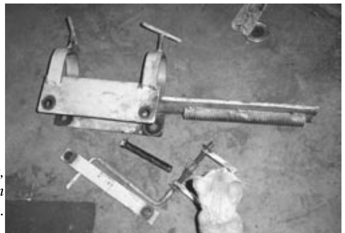
Left, recoil spring assembly mounted on ram. This keeps it from slamming home at the top of the stroke.
