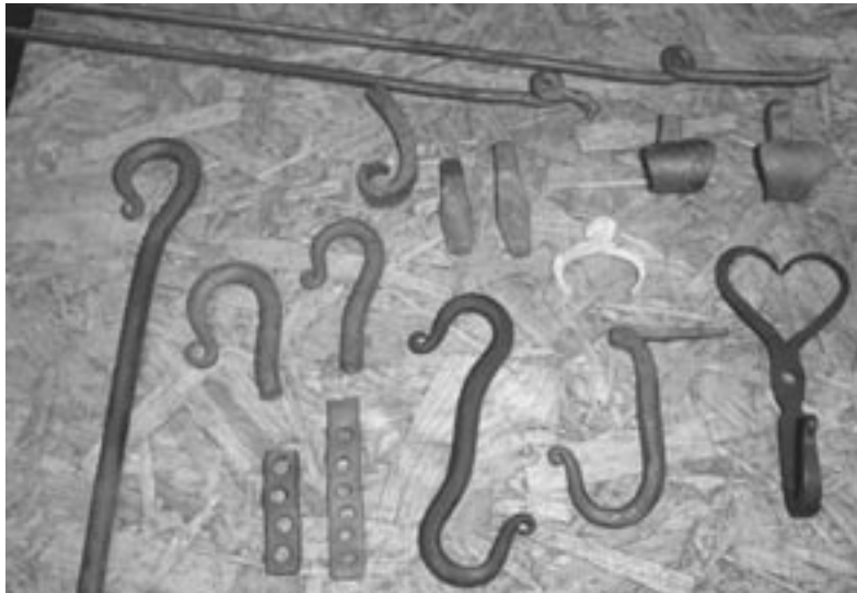
Week one projects, Simple hook ends, "S" hook, drive hook, heart hook. Hole punch practice pieces, I told them they had to do at least 4 holes before trying the heart hook. Flat scroll, fish tail scroll, screwdriver point tapers, and tong clips (various stages of completion).
