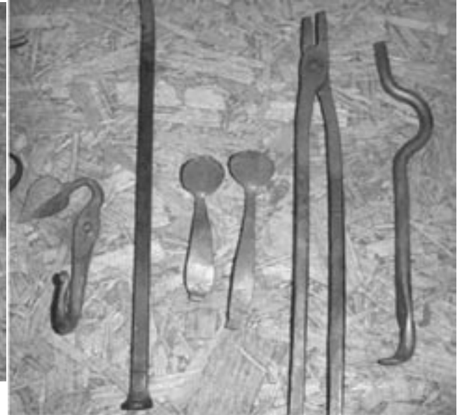
Week two projects, Leaf hook, half strike foot, half penny foot, flat jaw tongs, and the sample of the bolt tong jaws.
