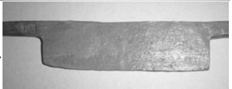
Above, rough forged blade Below, blade ground and hardened
