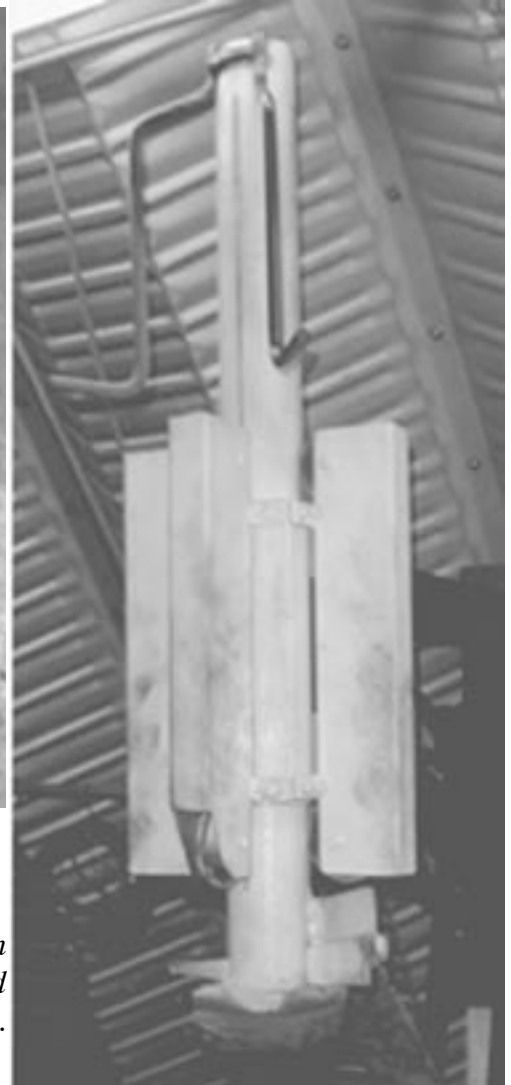
Right, Double pull down handles installed on finished ram in it's guides.
