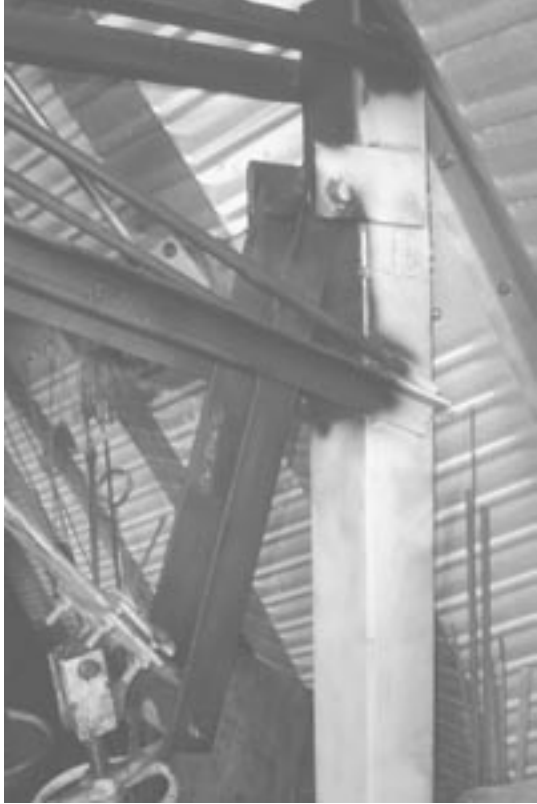
Above, Treadle control linkage. Below, worn out pivot bolt
