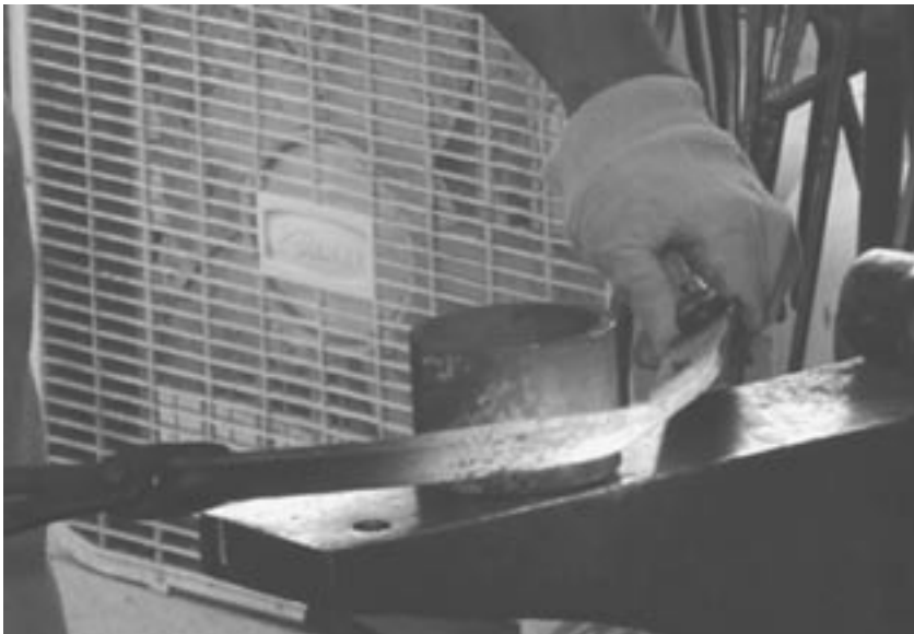
Bending the bar the easy way around the round form. The taper on the back, and slant on the sides just happens naturally because of the first bend.
