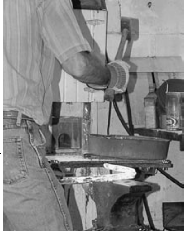
Folding over the steel to increase the layer count
