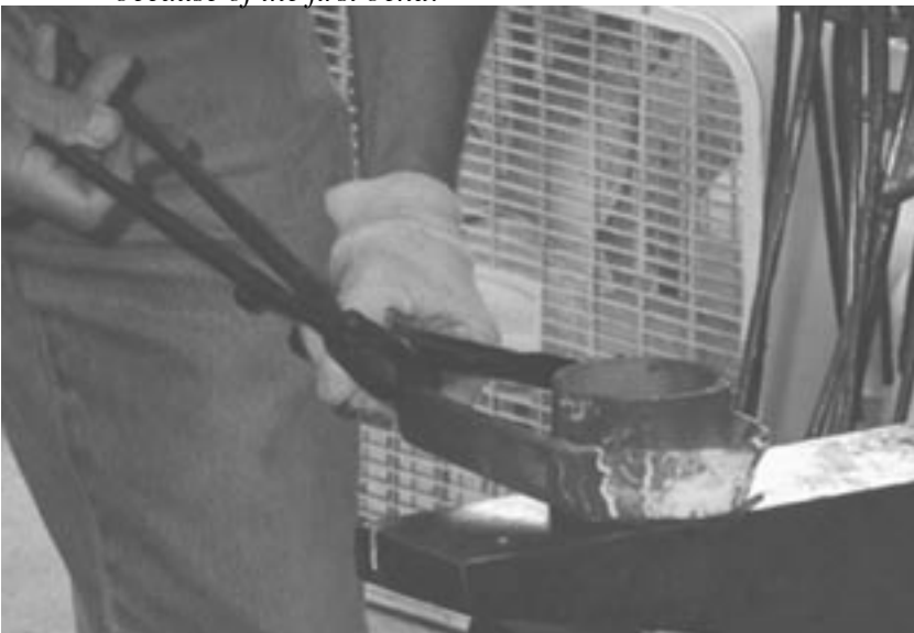
Bending the bar the easy way around the round form. The taper on the back, and slant on the sides just happens naturally because of the first bend.
