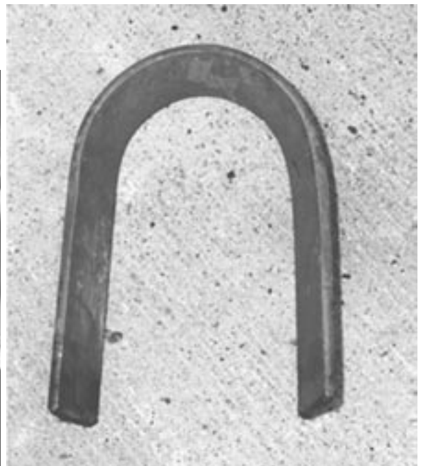
Below, the finished form. Make sure the slant on the sides have the same angle. A brace between the legs will be added later.
