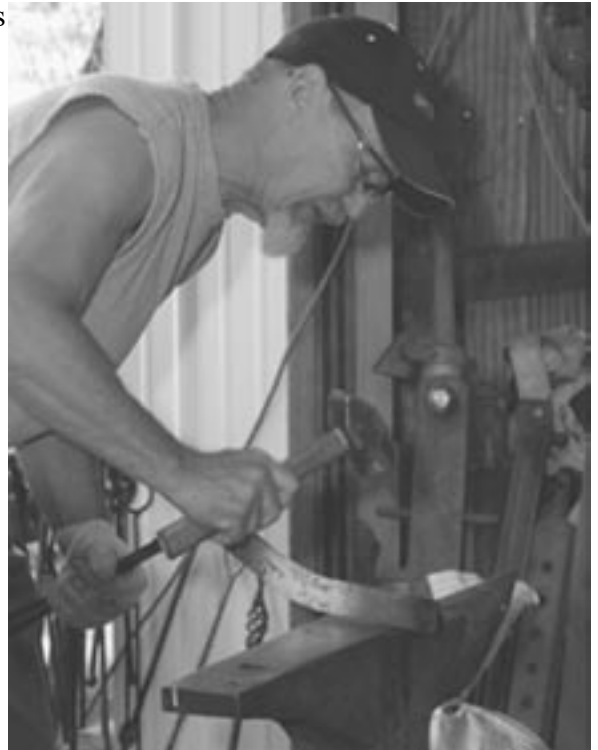
Above, bending the bar on edge to match your pattern.
