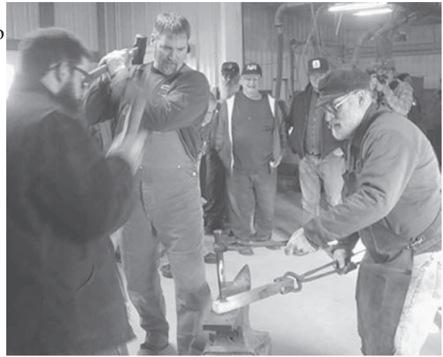
Driving the drift through
