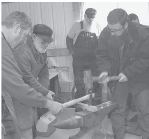
Hot Cut off main Bar
