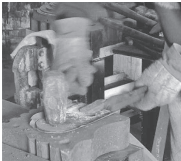
Don has a special tool to form shovel blanks in the swage block. It is a 1/2" thick plate welded to a pair of tongs. The
