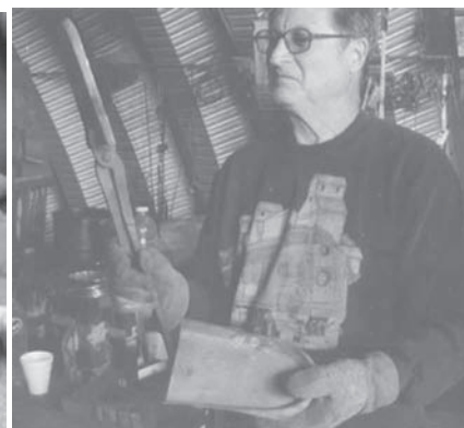
Don has a special tool to form shovel blanks in the swage block. It is a 1/2" thick plate welded to a pair of tongs. The
