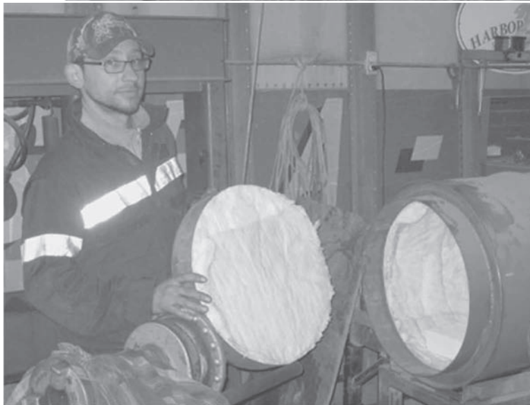
Sergi Roraback and his 55- gallon drum forge/heat treating oven, heated by acetylene rosebud torch
