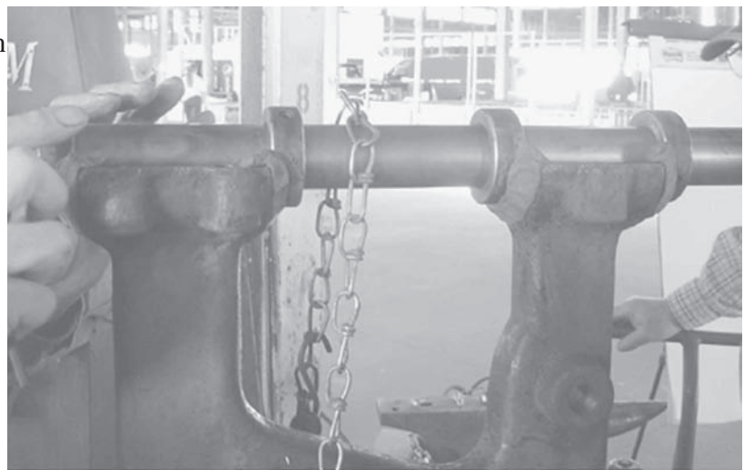
Shaft with collars and putty in place
