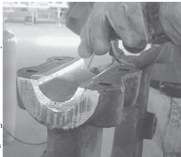
Lower bearing after cleaning up.
