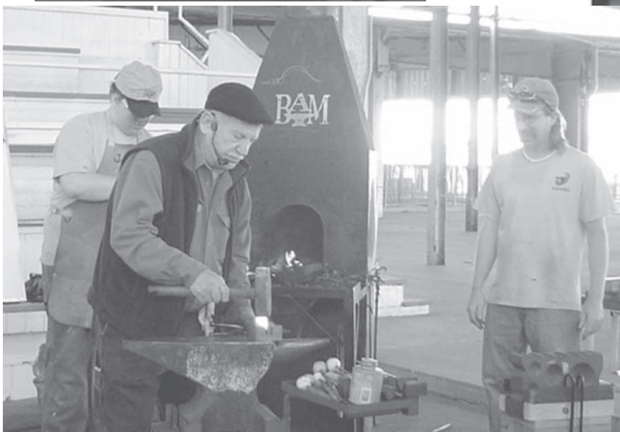
Left, Lou upsetting the edge of a flat bar.
