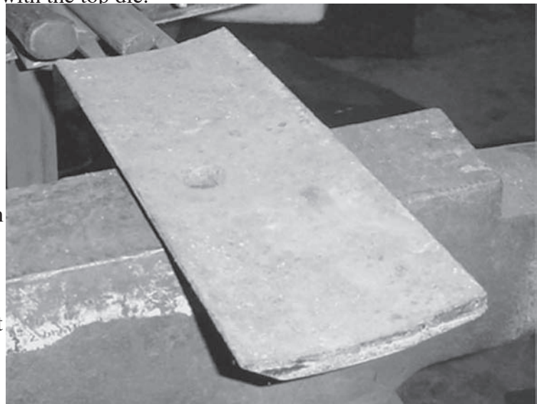
Grader blade before straightening.
