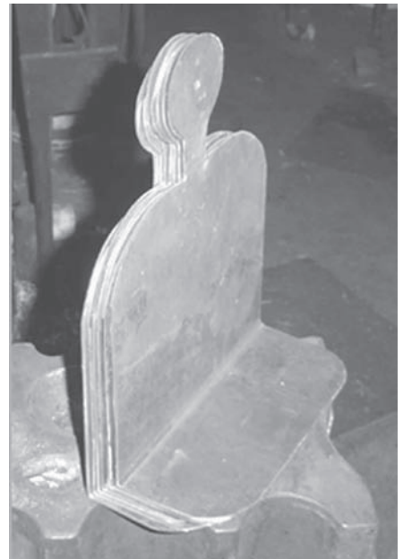
The beauty of the brake is repeatable results. I made several parts and they all came out the same.
