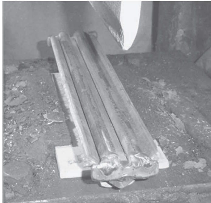
The close bend adapter made from 1/2" rd. just drops into place when needed.
