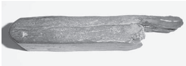
Block of damascus after welding and folding
