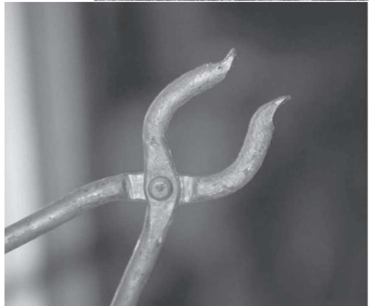
The rivet set is made with the same ball punch that was used to make the head impressions in the bolster.
