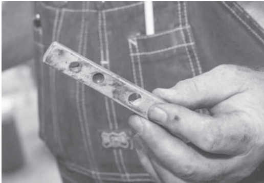
Close up of bolster, two rivet head impressions and a through hole.
