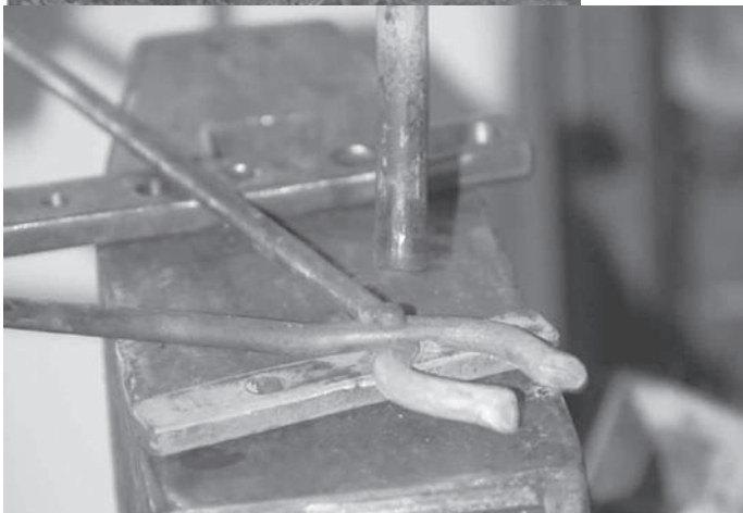
The rivet set is made with the same ball punch that was used to make the head impressions in the bolster.
