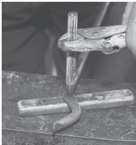
Close up of bolster, two rivet head impressions and a through hole.
