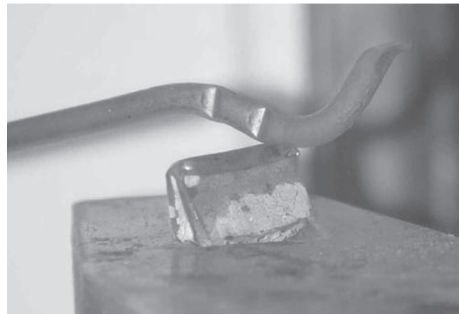
Above, fuller the area for the joint.
