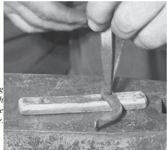
Punch first side of hole with flat end punch.
