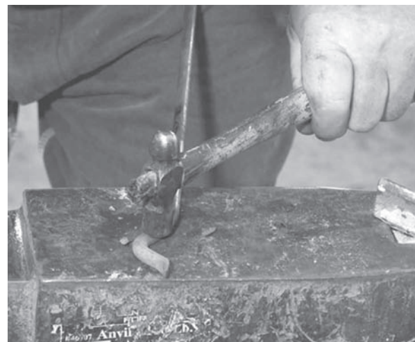
Left, check the fit of the two pieces before punching the holes.
