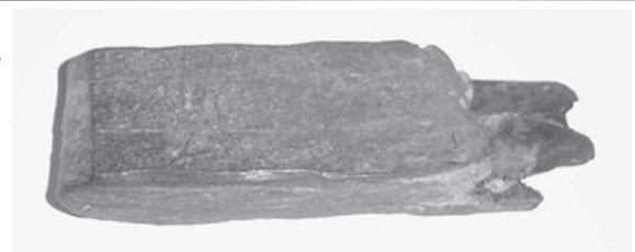
Block of damascus after welding and folding
