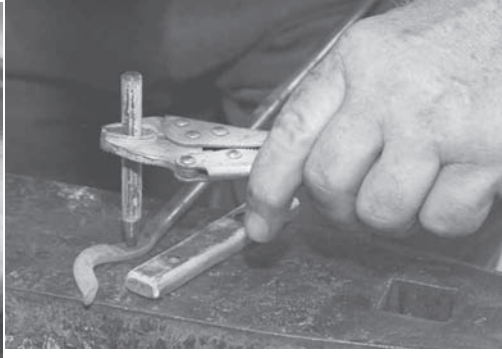
Punch first side of hole with flat end punch.
