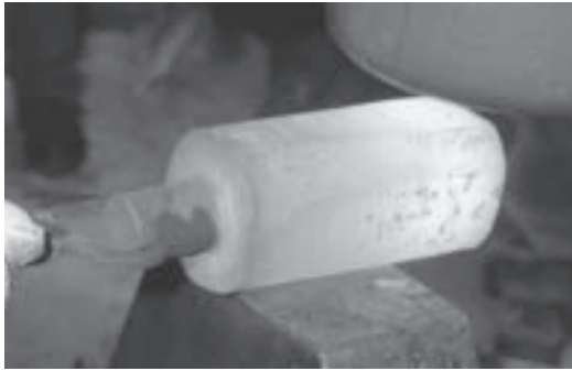
On the 400lb Chamberburg -Square up shaft, draw out and cut off a chunk with hack.
