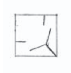
Figure 3 Make chisel marks where shown above
