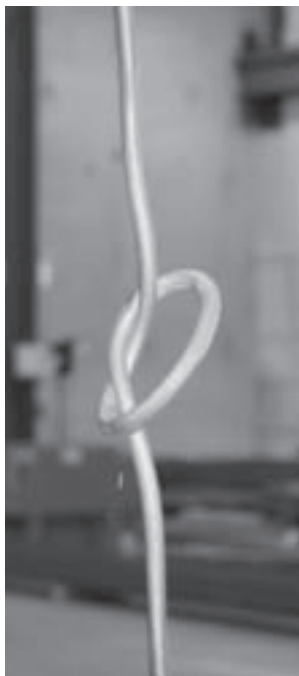
Picture to the right shows how much material Phil started with to tie the knot in the 5/8" bar.
