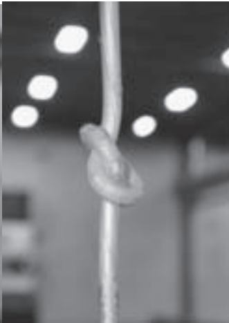
Picture to the right shows how much material Phil started with to tie the knot in the 5/8" bar.
