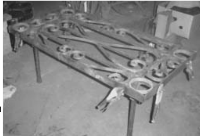
Fitting the scrolls into the frame as we made them.
