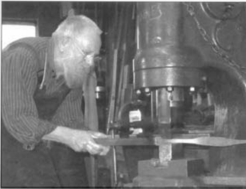
Paul at the power hammer. Note he is using slightly curved drawing dies.
