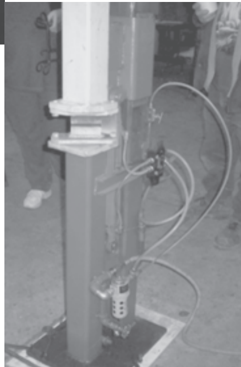
Bellow, Don Nichols' home made power hammer. The air cylinder is on the bottom which reduces the size of the frame considerably.
