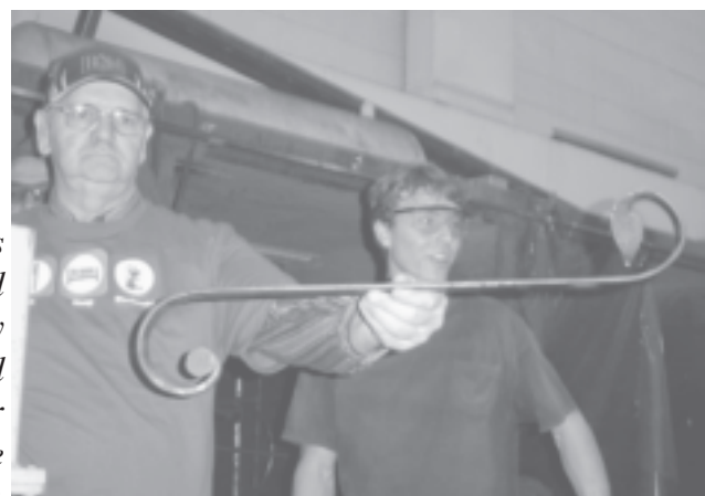
Right, Don holds up the finished bar with a penny scroll on one end and a blown over leaf scroll on the other.
