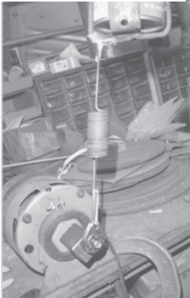
Above, close up of the eccentric and connector. Initially I just had the spring hooked on a bolt. The bolt quickly wore out (10 cans), I had this small roller bearing which worked out great.
