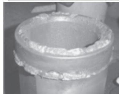
Pictures of piston/ram before repair
