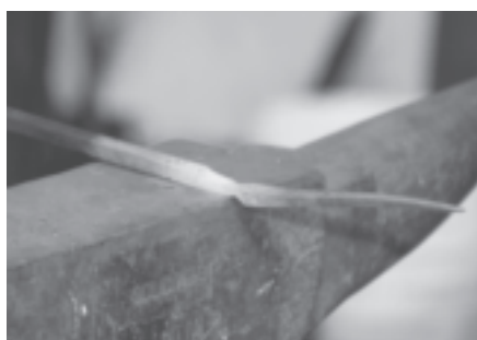
Draw a long taper, section off between leaf and stem.
