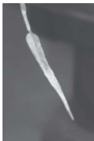
Flatten the leaf. (left) Use simple tool and small hand held fuller to make vein down the center.
