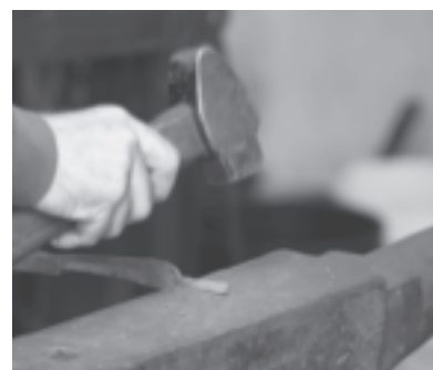
Cut loose from main bar, forge stem to shape.
