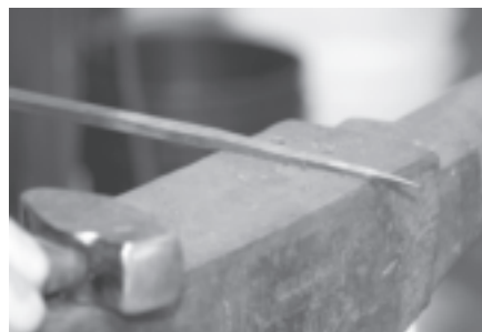
Draw a long taper, section off between leaf and stem.
