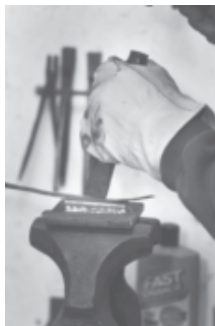
Flatten the leaf. (left) Use simple tool and small hand held fuller to make vein down the center.
