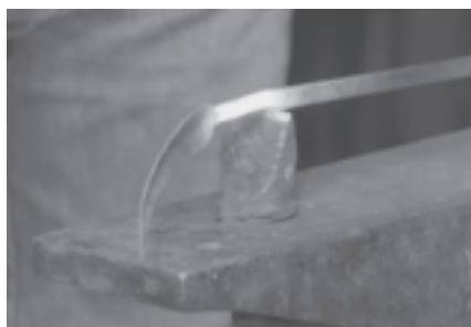
Cut loose from main bar, forge stem to shape.
