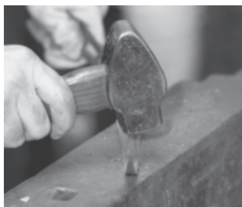
Roll the sides of the leaf out by gently tapping the spine, while the edges are in contact with the anvil.
