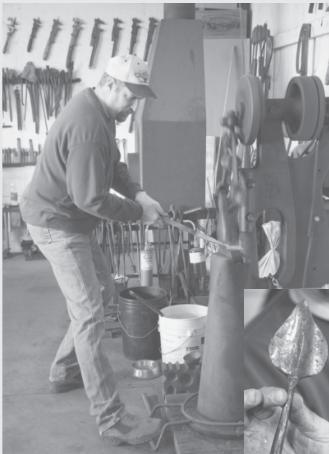
Ken Jansen makes a leaf under the power hammer.
