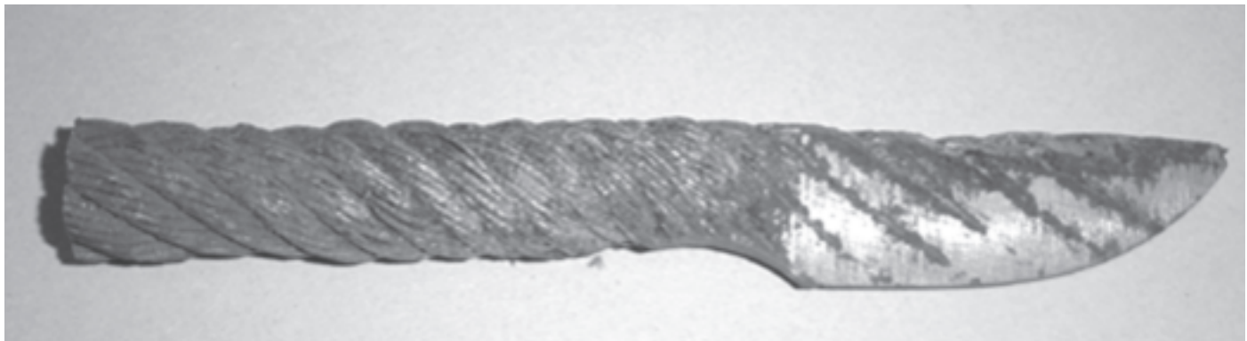
Daniel's cable damascus blade. It's kind of rough, but he was mainly demonstrating technique and not going for a finished product.
