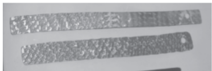
Above, Texturing tool made by welding three pieces of re-bar to a flat plate. Below, a sample of what a hot bar looks like after it is driven into the tool under the power hammer. (on display at Ned's meeting)
