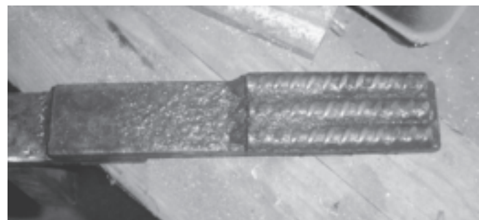
Above, Texturing tool made by welding three pieces of re-bar to a flat plate. Below, a sample of what a hot bar looks like after it is driven into the tool under the power hammer. (on display at Ned's meeting)
