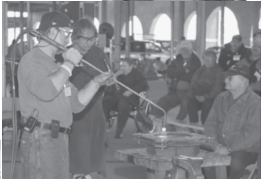
Below, Michael makes a large disk from a large billet of copper. Right, after clamping the disk in a fixture, Joe heats it with a torch for Michael to sink unto a bowl.
