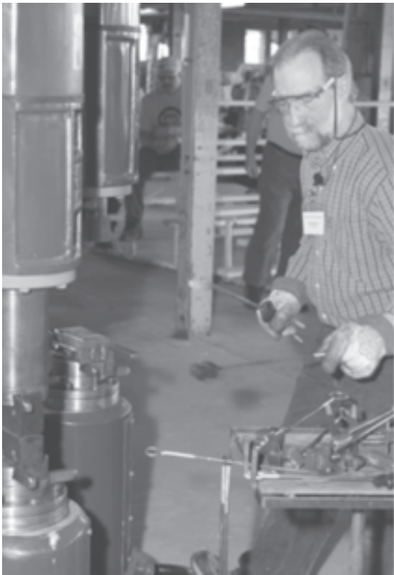
Below, Michael makes a large disk from a large billet of copper. Right, after clamping the disk in a fixture, Joe heats it with a torch for Michael to sink unto a bowl.
