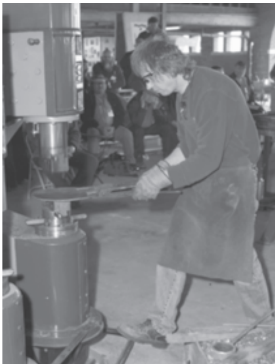
Below, Michael makes a large disk from a large billet of copper. Right, after clamping the disk in a fixture, Joe heats it with a torch for Michael to sink unto a bowl.
