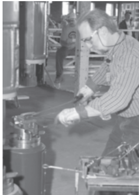
Joe showed how he does most of his work under the power hammer using hand held tools and jugs clamped to the bottom die.
