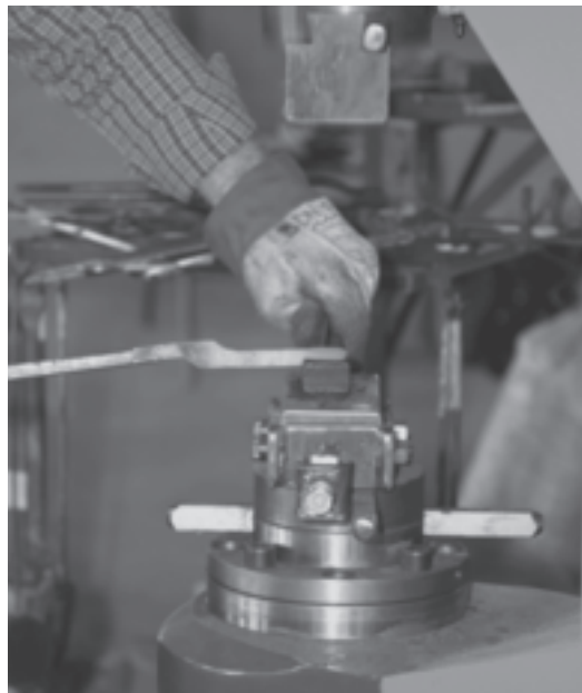
Joe making tongs under the power hammer.
