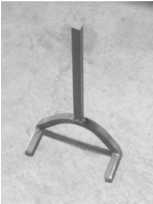
Safety Device made from 1/2" square stock.
