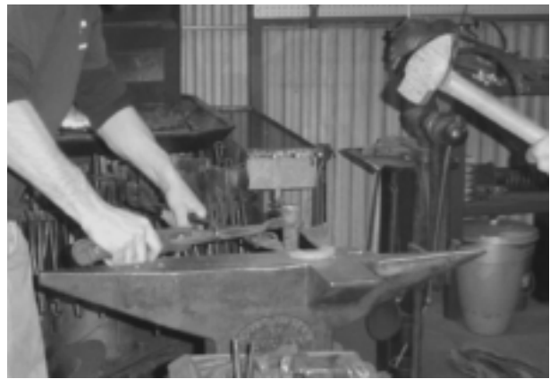
Fuller around body to create a ridge.
