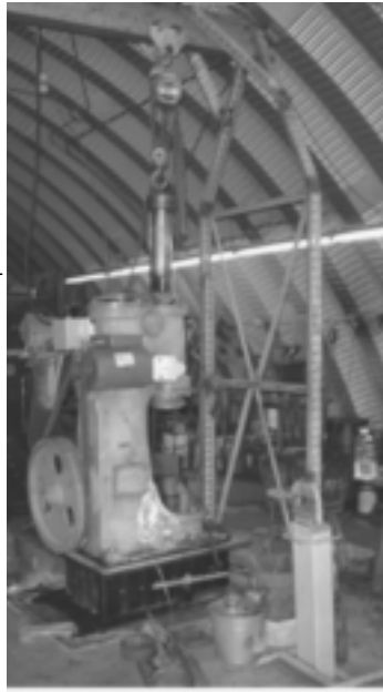
Pulling the ram for cleaning. Also shows the construction of my crane.
