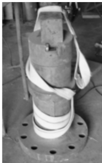
500 lb. anvil made from a large axle with flange.
