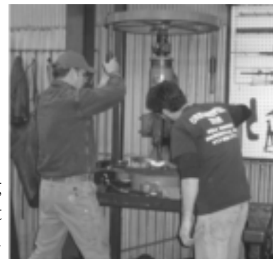
Bending body using the press and a set of blocks.
