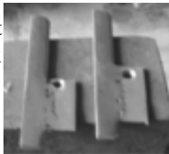
Fixture to protect ram guide slot while honing.
