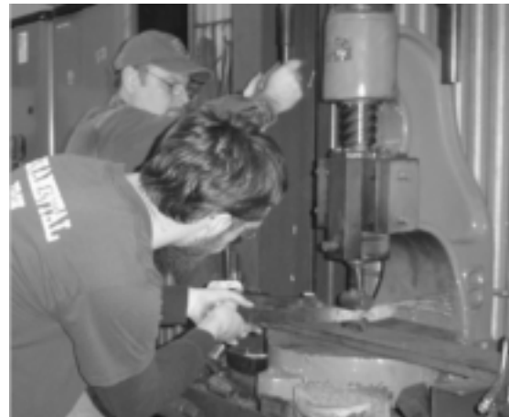
Use press to draw out second tail fin.
