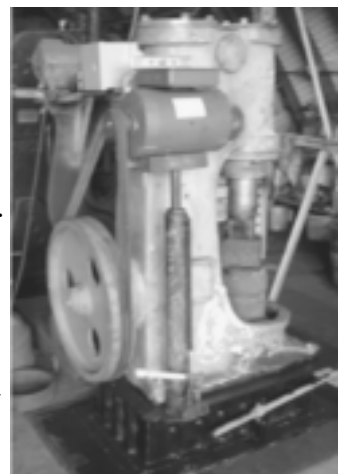
Using a hydraulic jack to tension the drive belts.
