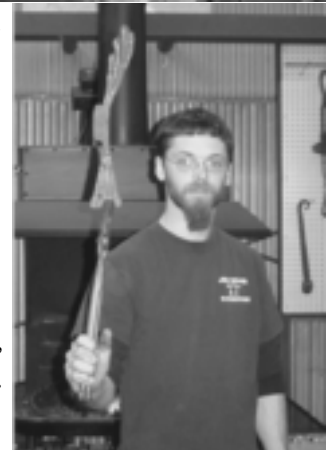
Use press to draw out second tail fin.
