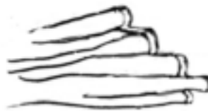
Use a fuller to create a ridge at each of the steps.
