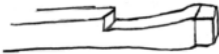
The first step is to butcher off material for the first fin.
