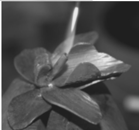
The petals are then heated and shaped with scrolling tongs.
