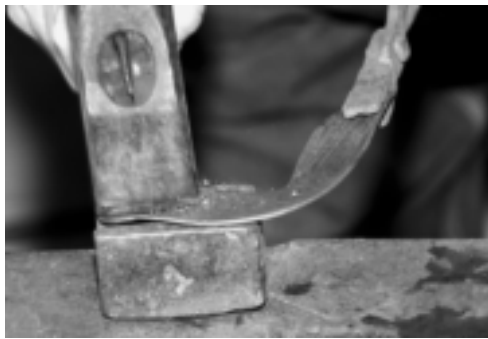
Shape the leaves and petals on a small swage block
