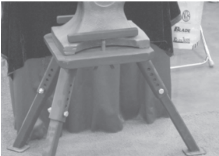
Pictures of Anvil Base and Tool Stand Base sent in by Mike Gentsch, the pads on the tool stand are tapped so that the stand can be levelled.
