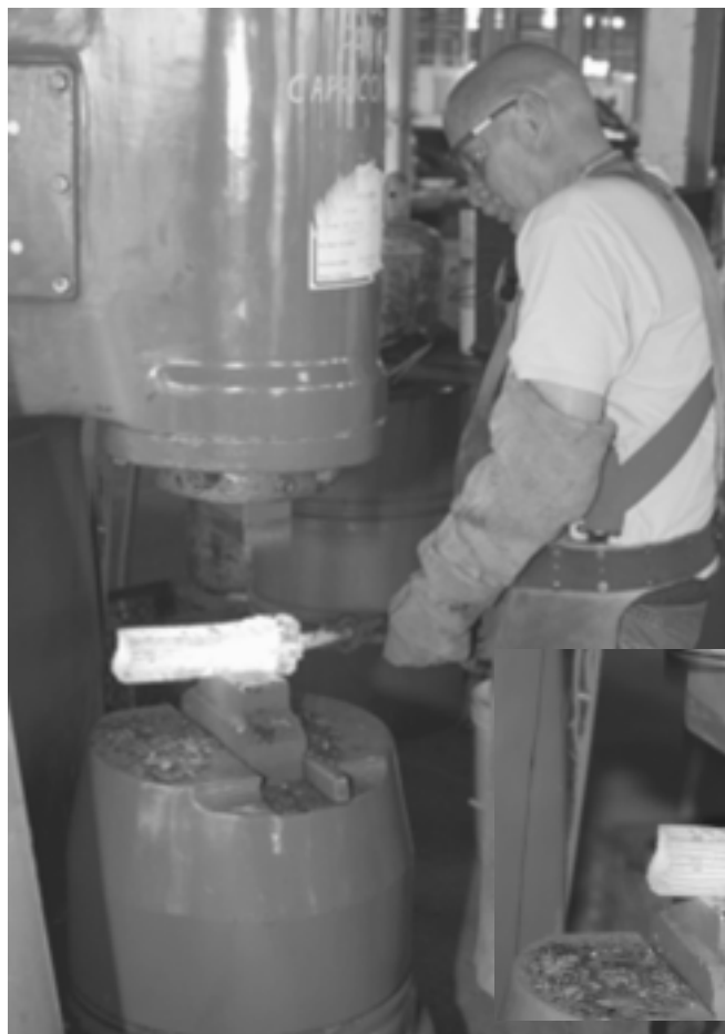
Making the initial weld.
