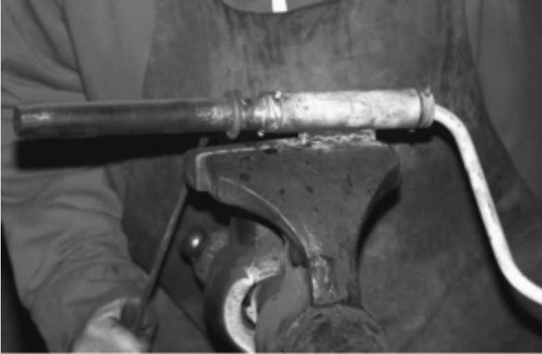
Winding jig is just two pieces of pipe with a handle to turn the inner pipe.
