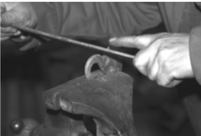
Cleaning up the handle to blade transition
