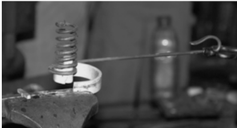
Winding jig is just two pieces of pipe with a handle to turn the inner pipe.
