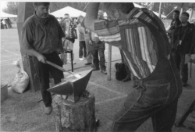
First, a blunt taper was forged on the end of a square bar.
