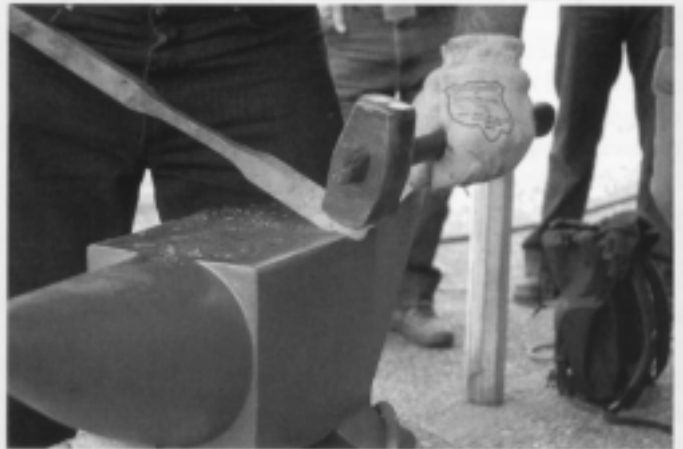
...then move to the far edge. Brian used a broad fuller, making half-faced blows.
