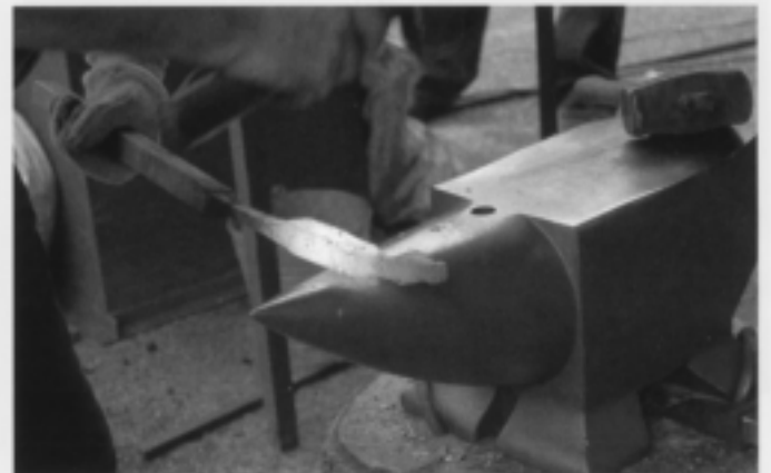
Chisel in the suggestion of a mane before you curve the neck. A wooden mallet is good for coaxing the neck into a curve.
