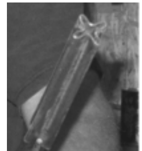
Tubing after collapse
