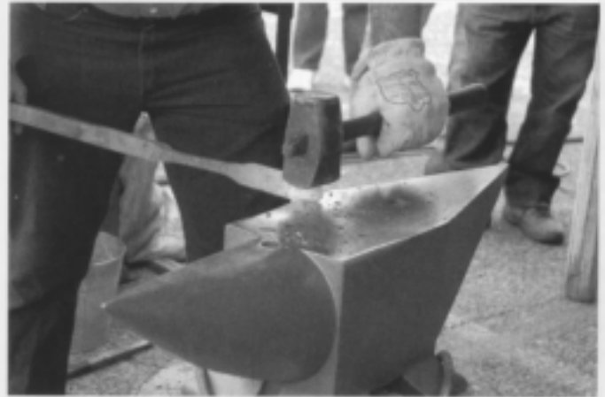
Notching the cheek. First at the near edge of the anvil...
