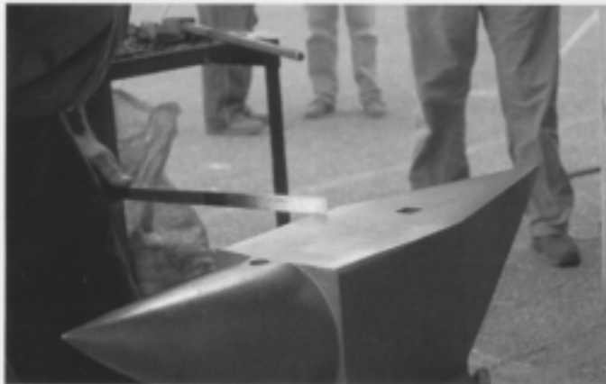
Starting a seahorse by forging a nose.
