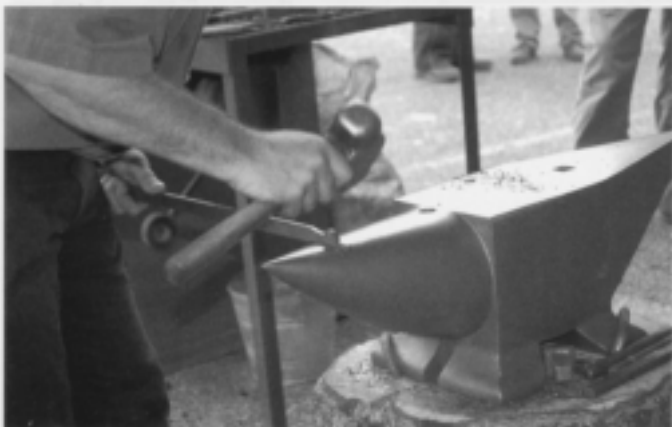
Rounding off the "tab" that will become part of the head.
