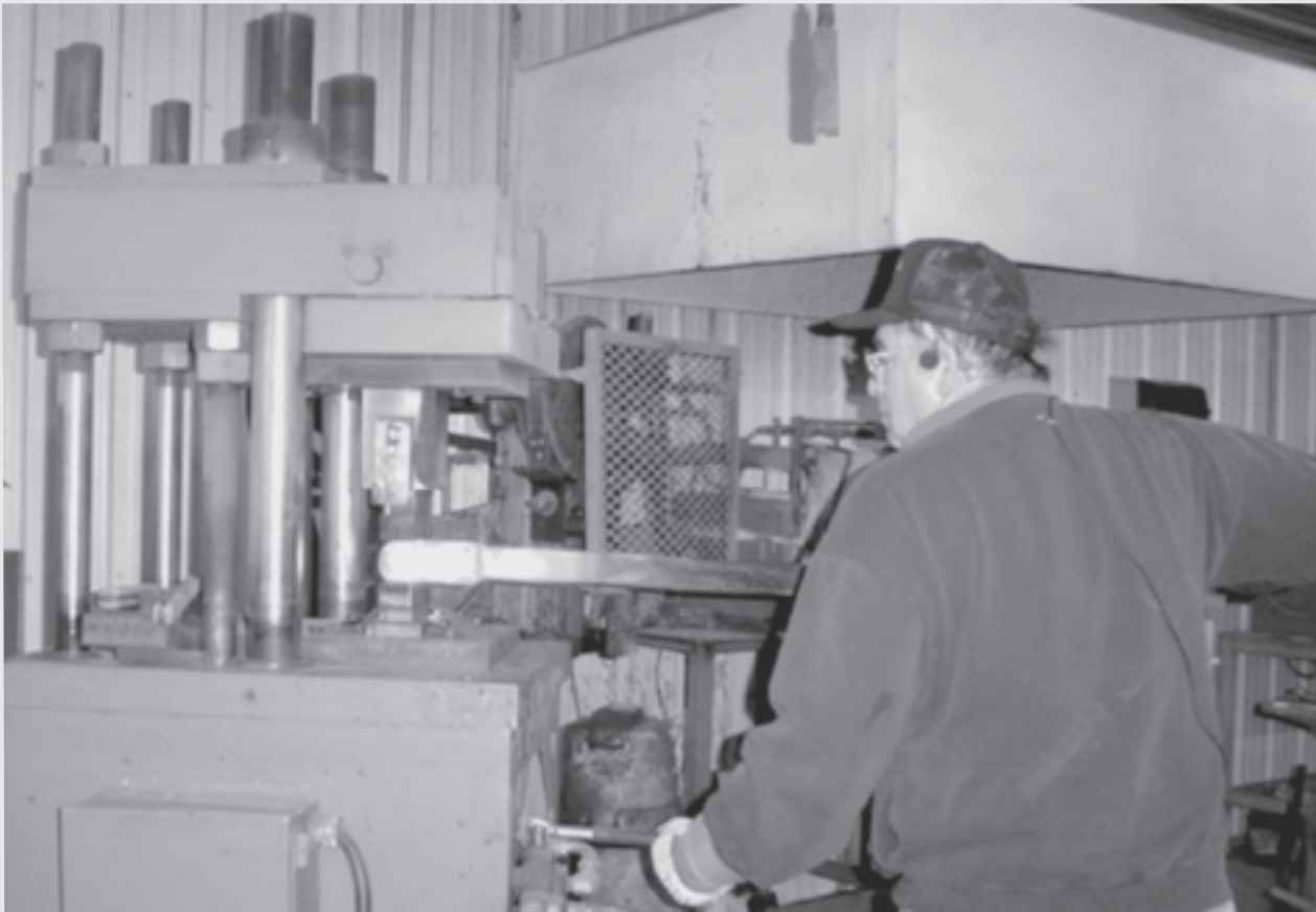
Tom McGinnis Welding a Powdered Metal Canister under the press
