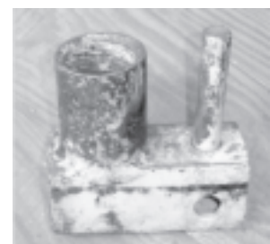
Bending jig. 1.5" pipe and 1/2" bar welded to a piece of 1.5"x1.5" angle iron.
