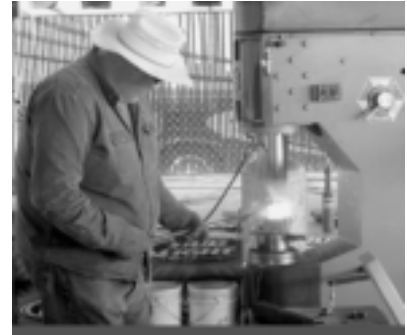
Stick the weld by hand and then draw it out on the power hammer.
