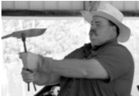
Checking straightness before grinding
