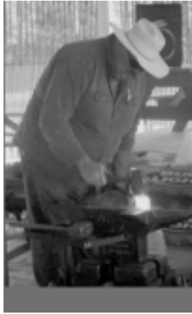
Stick the weld by hand and then draw it out on the power hammer.
