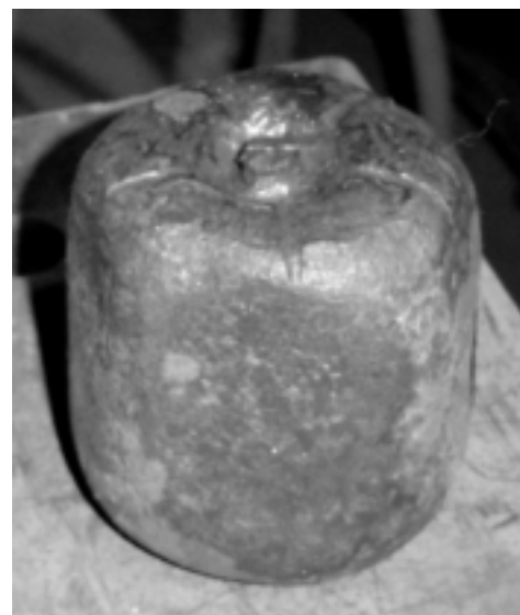
Apple bottom showing Nub, Flats, and fullering.
