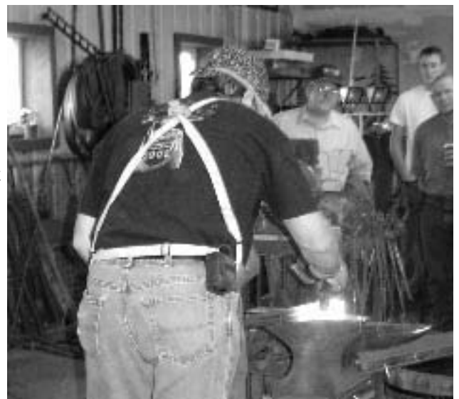
Kirk Making initial weld by hand
