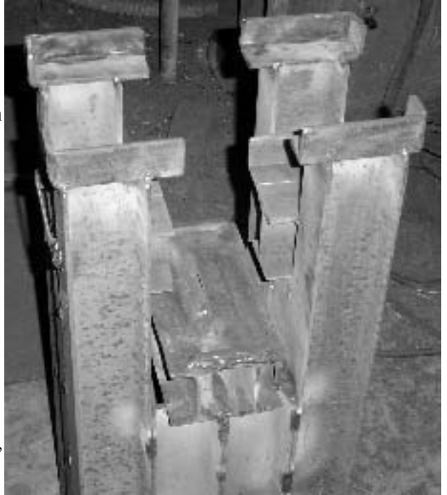
Empty Swage Stand shows the three working levels and construction.
