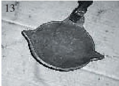
13 ladle 013--What the pourspouts look like after the initial forming.
