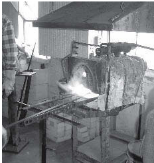
Corbin's Forge, Three billets at once
