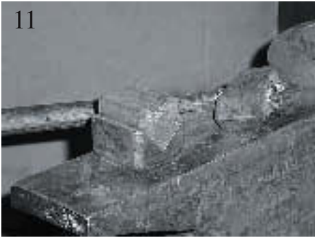
11 ladle 011--My bottom V swage in its base. There are 4 different sizes 1 to each side. The block lifts out so it can be rotated, there are also round swage blocks that fit in this base.
