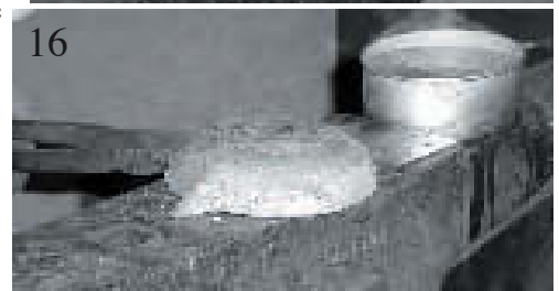
16 ladle 016--The ladle laid upside down on the anvil to flatten the pourspouts by tapping on the spot cooled bottom.
