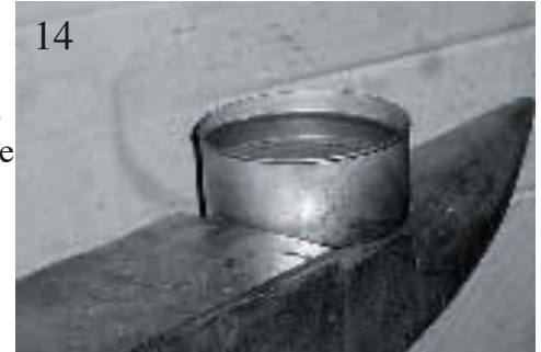
13 ladle 013--What the pourspouts look like after the initial forming.
