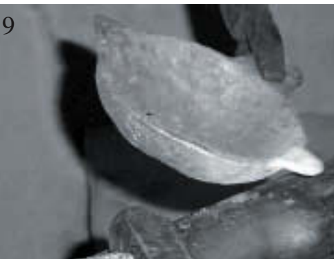
ladle 009--Working the pourspouts down.
