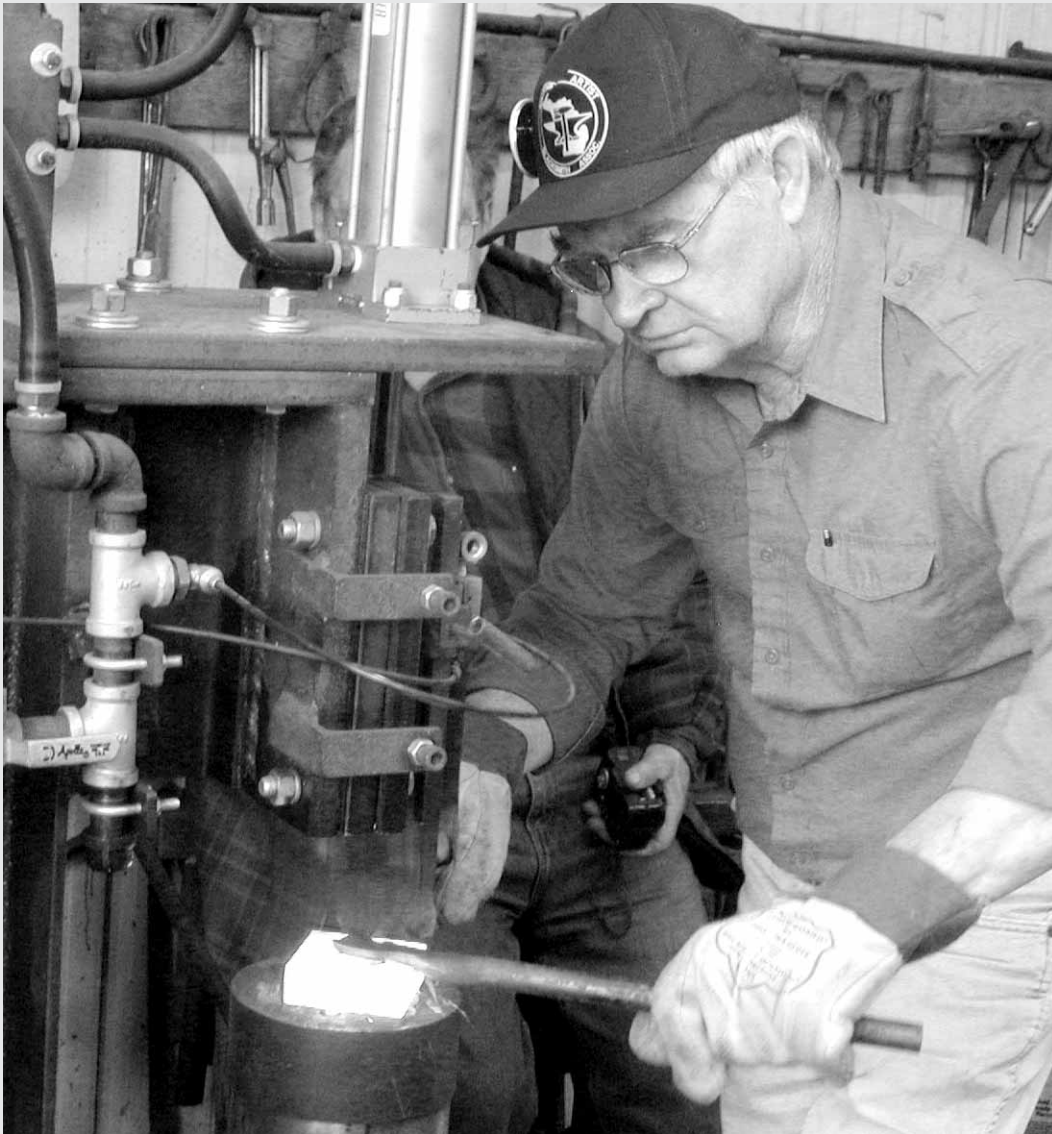
Maurice Ellis demonstrating making an open die
