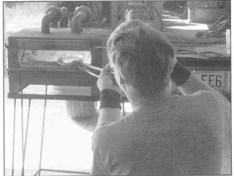
Neal checks his shoe in the gas forge.
