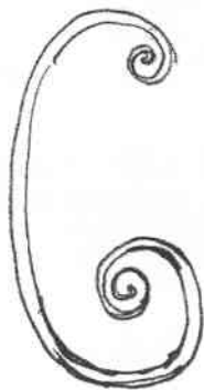
EXISTING SCROLL MEASURED BY STRING
